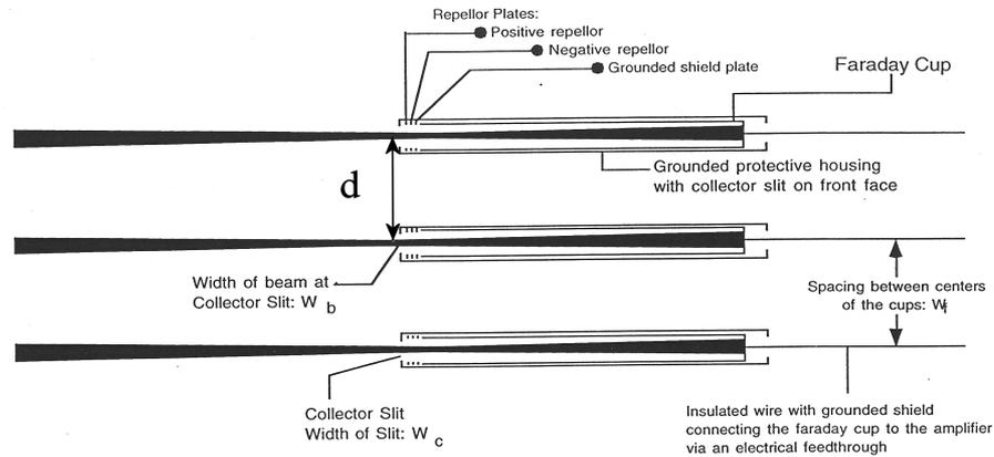
Figure 2: Diagram of three faraday cup collectors set for Sr<sup>87</sup> in the axial position) for a mass spectrometer with an effective radius of 54 cm. Scale: 4x. Ion beams are diverging with half-angles of 1°
