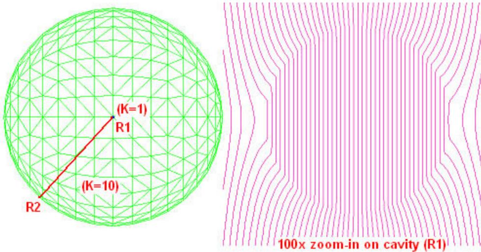
A cavity of radius 0.05mm exists at the centre of the dielectric cylinder.
