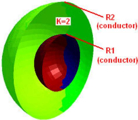
This is modeled with four shapes. The first two shapes are the inner and outer conducting spheres, respectively:
