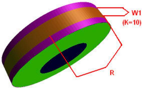
A circular disc of radius 0.5mm is at  $z = -0.1\text{mm}$ , at  $-0.5\text{V}$ . A similar disc is at  $z = +0.1\text{mm}$ , at  $+0.5\text{V}$ . The number of segments in each of these discs is 96. The inaccuracy used for evaluation of the fields at the dielectric interfaces is 0.001 (but see below).
