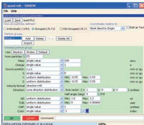
**Particle initial conditions** can be defined in various ways. The “FLY2” format in SIMION allows quick definition of many types of particles random distributions and sequences. Particles may also be exhaustively enumerated (optionally imported from a text file).
