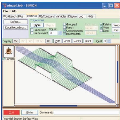
**Viewing of the system is highly interactive,** allowing adjustment of parameters and viewing of the system even during particle flight (trajectory calculation). SIMION supports cutting away volumes to see trajectories inside, zooming, viewing potential energy surfaces, contour lines, and trajectories, and reflaying particles as dots for movie effects.
