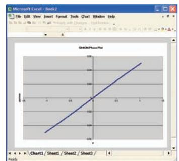
In the example above, trajectories are calculated while phase space data is interactively plotted in Excel via the Lua COM interface
