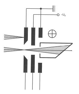
Magnetic field plus repellor plate reduces secondary electron loss to a few hundred parts Per million or less
