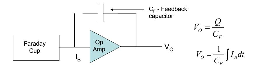
More sensitive than CVC, a 100fF capacitor and 10<sup>-17</sup> A beam gives a 0.1 mv/s voltage change (same current even with 10<sup>12</sup> ohm resistor gives 0.01 mv voltage output
